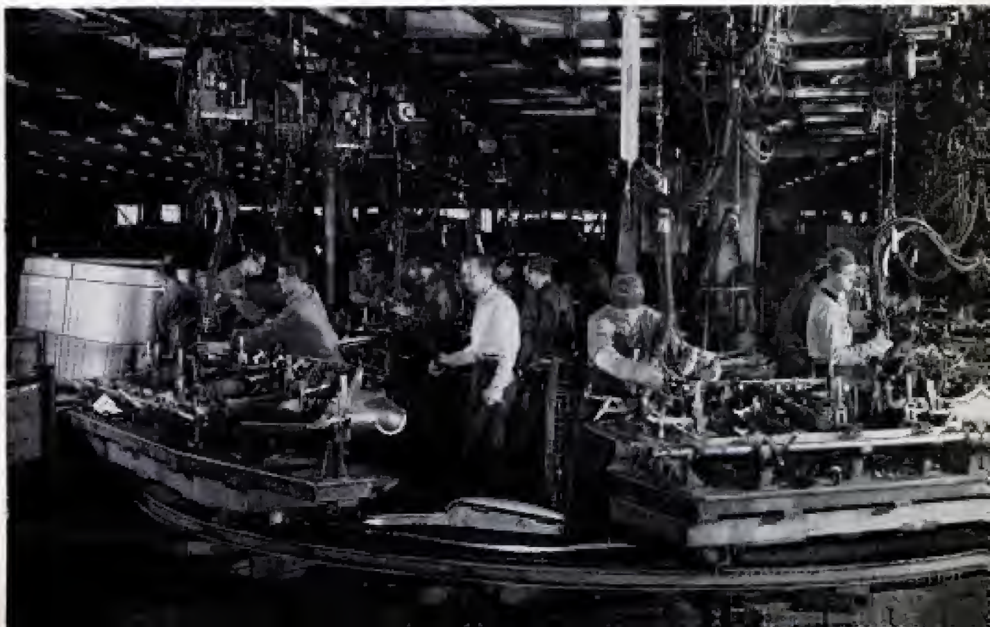
Automation aids car-body workers by holding and moving the steel panels and moving the tools into position
